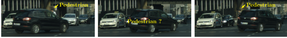
Figure 3: Sequence of temporarily occluded road users [11].
