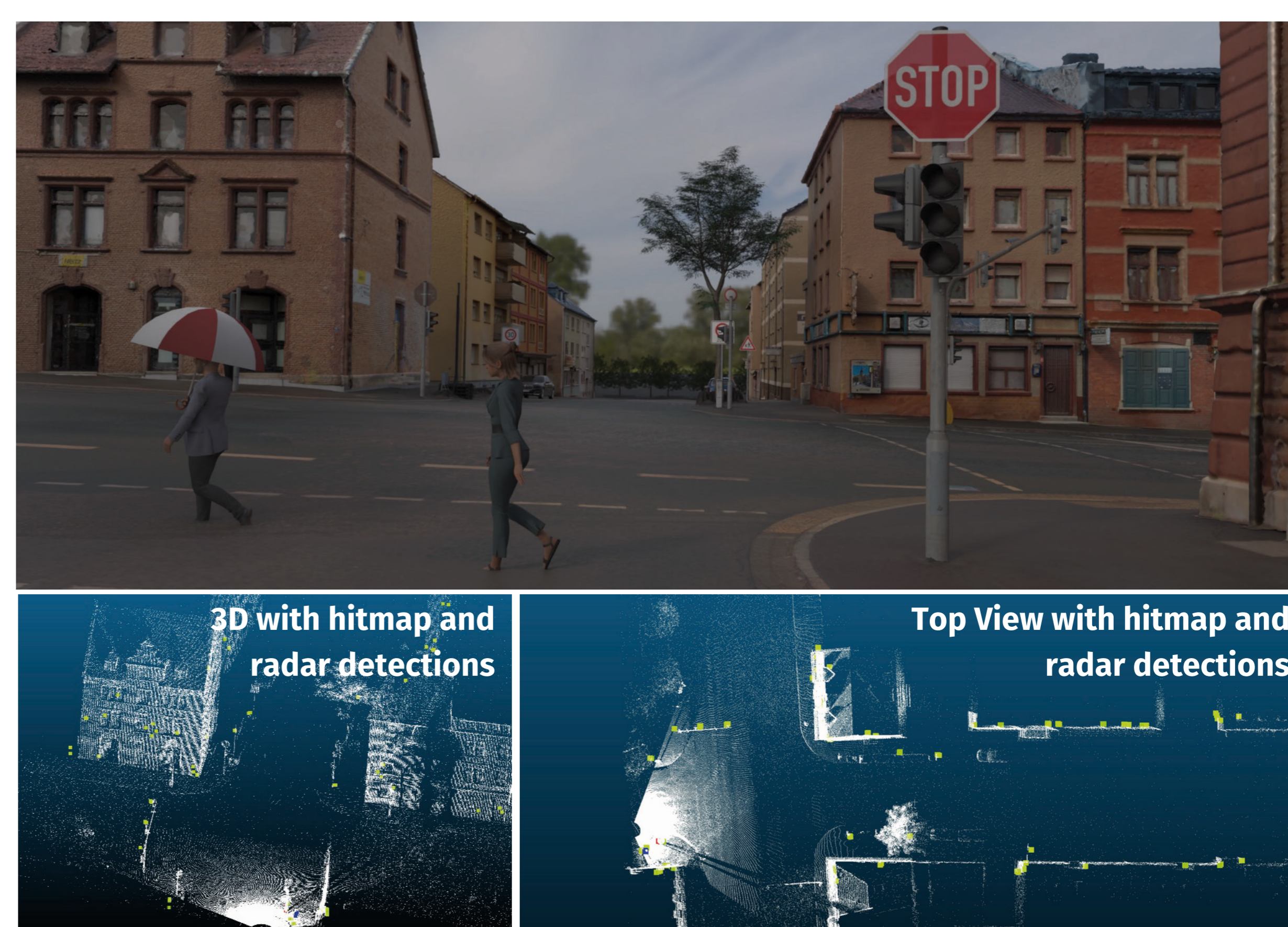
Figure 6: Rendering of Urban intersection scene including RGB (above) and radar point-clouds with path-tacer hitmaps (below) ©BIT-TS
