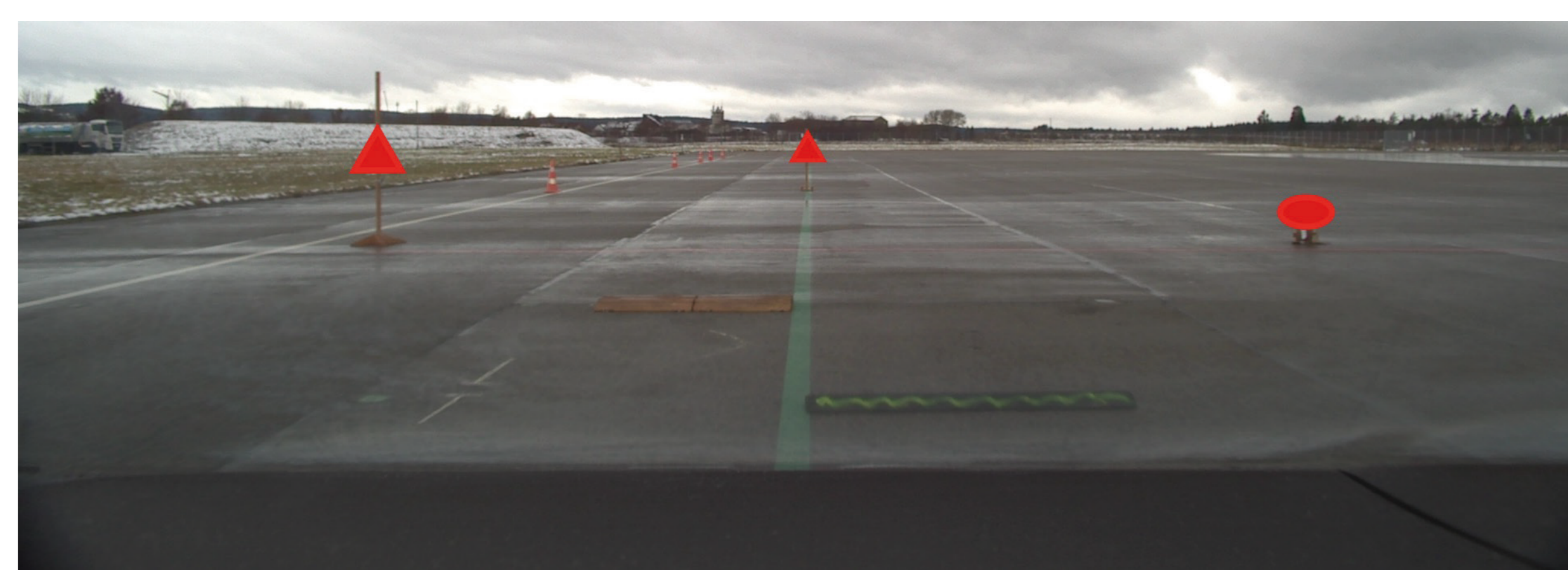
Figure 1: Test Measurement at test site in Renningen with radar reference targets ©BOSCH
