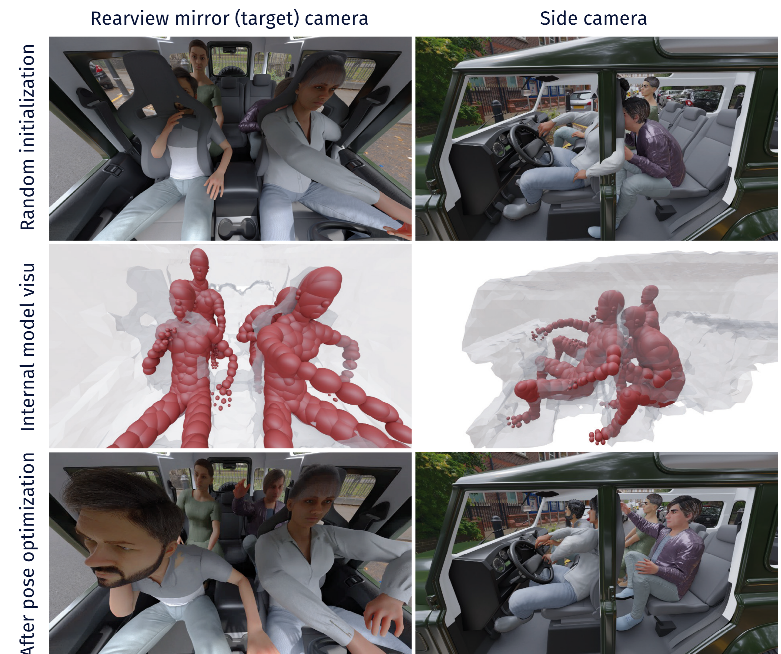
Figure 3: One example of virtual human creation and pose adaptation in a 3D vehicle environment; down left is the final image (© Bosch)
