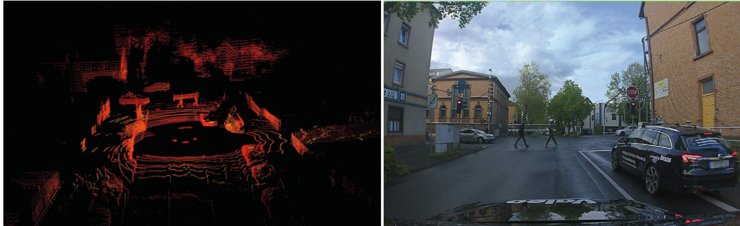
Figure 3: Example of scala cloud and camera image from Aschaffenburg recording campaign (© Valeo)
