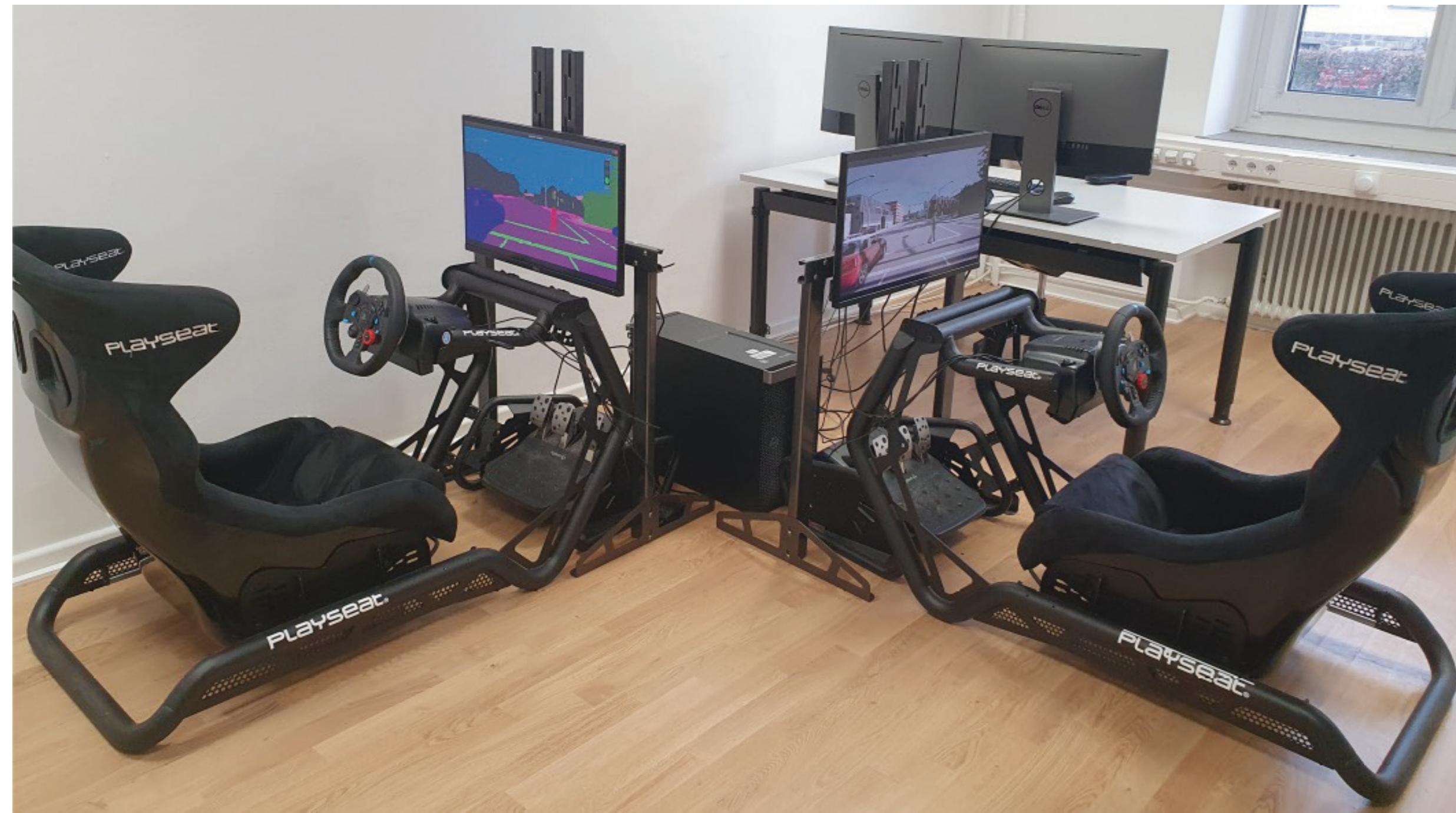
Figure 1: Test rig including steering wheels, pedals, seats and screens, where two human drivers can control the ego-vehicle.
