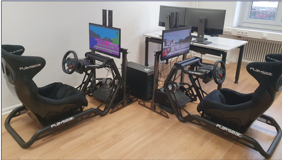
Driving simulator including steering wheels, pedals, seats and screens.
