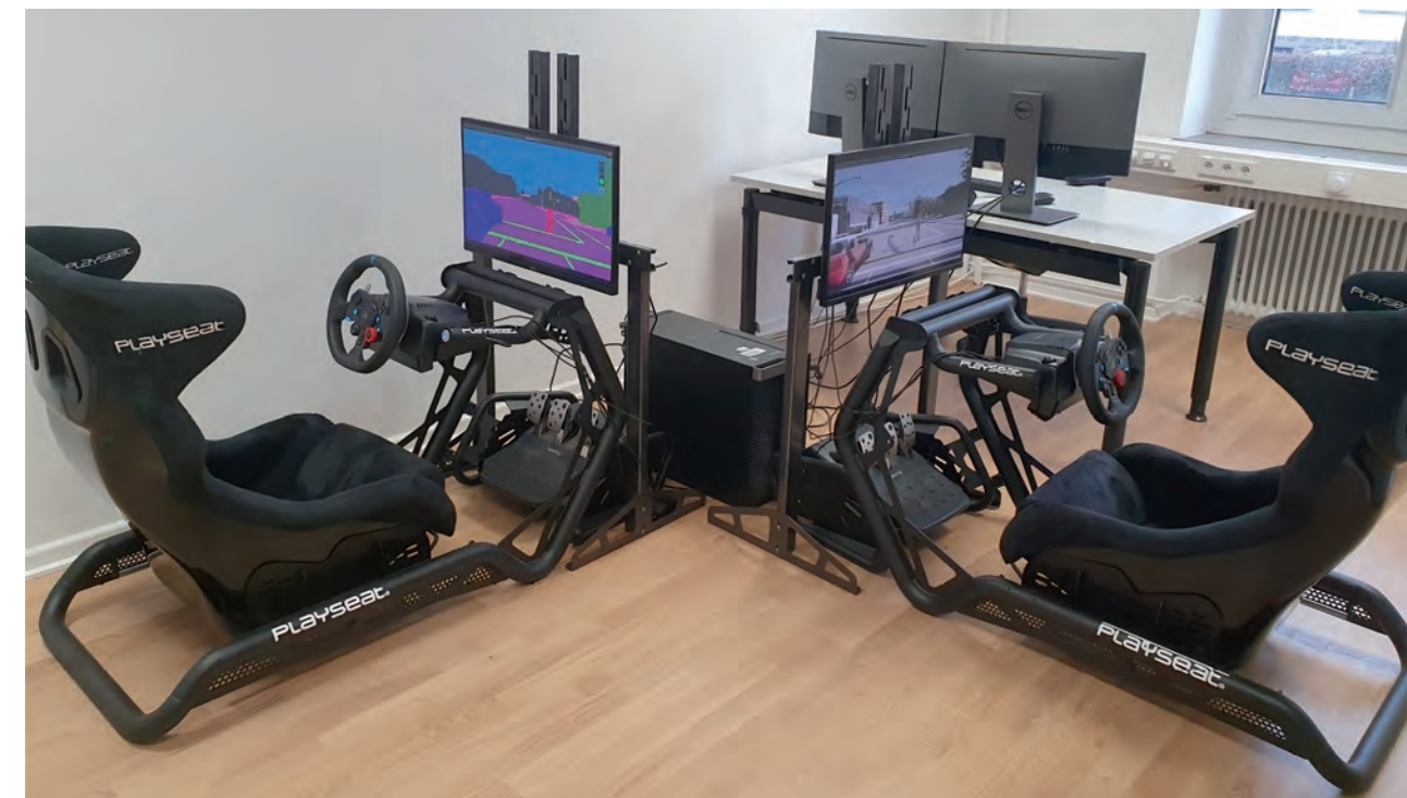
Figure caption: Test rig including steering wheels, pedals, seats and screens.
