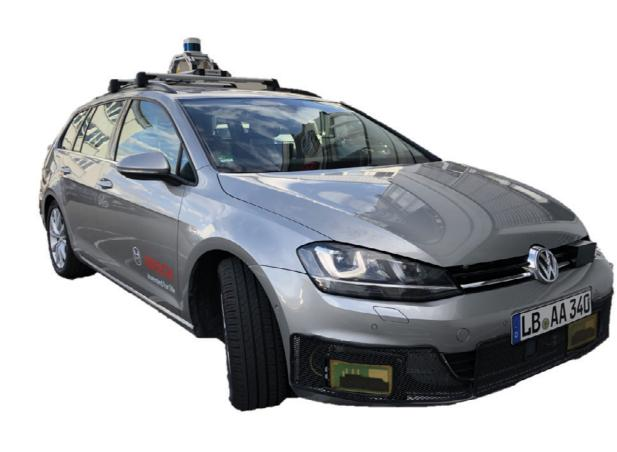
sensor raw data for the KI Data Tooling dataset. Each of the three vehicles is equipped with video cameras, one or more LiDARs and an inertial navigation system. AVL's vehicle is equipped with its own roof top box, consisting of 4 cameras, 3 LiDARs and an IMU. Bosch and Valeo additionally use their respective radar sensors.
